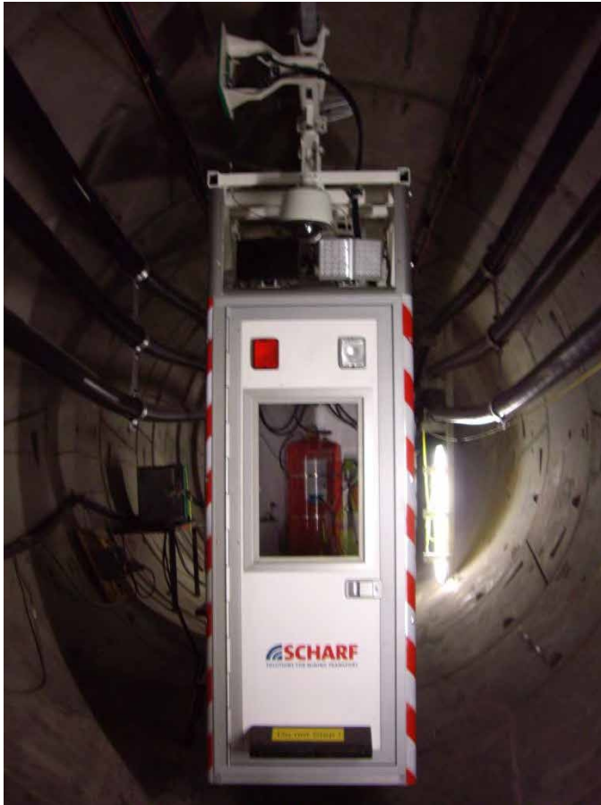
Figure 70 – Tunnel vehicle suspended from monorail
