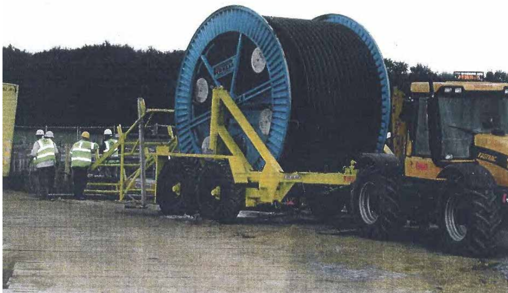
Figure 38 – Cable drum carrying trailer
