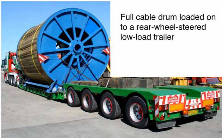
Figure 39 – Cable drum loaded transversely onto a trailer
