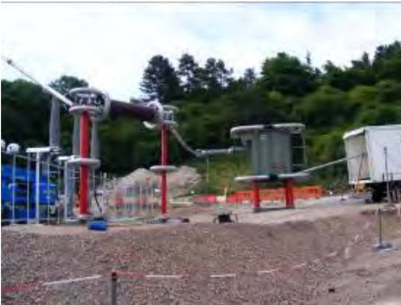
Figure 26 – Cable AC test voltage equipment
