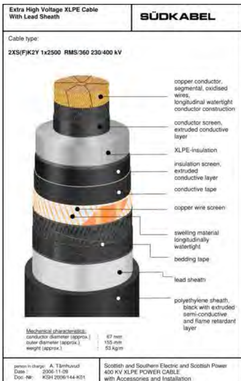
Figure 18 – Diagram of a 400kV transmission power cable
